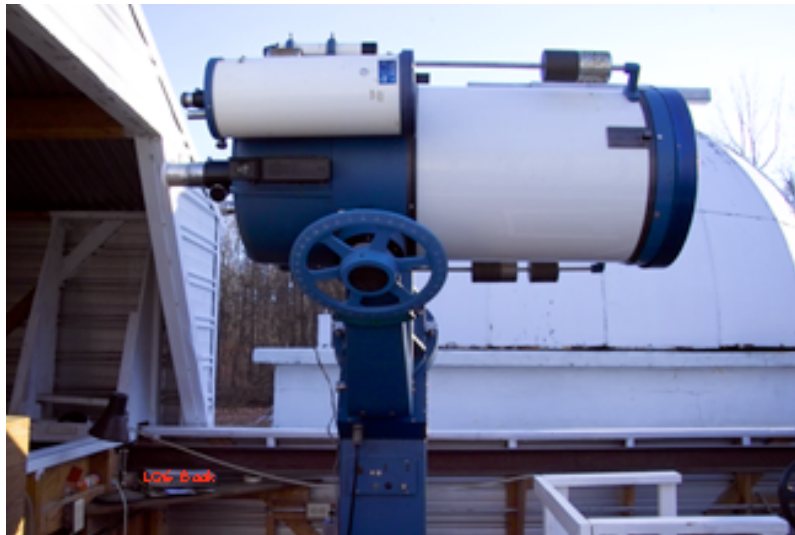
CI6 in proper stowed position for closing roof. Note the position of the fork aligned with base.
