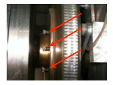
Picture 3: Dec. Clutch Adjustment Screws
