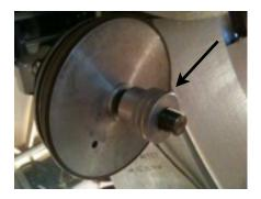
Picture 1: R.A. Clutch Adjustment Knob
