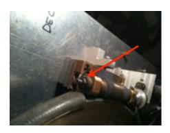
Picture 4: Dec. Worm Gear Adjustment Allen Screw
