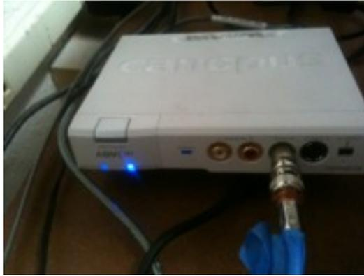
*Picture 1: ADVC Blue Light shall be on Analog (right)*
