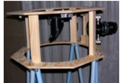
The cage framework, together enough for a focus test.
