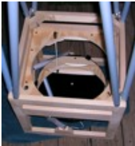
The completed mirror box framework, a collimation knob and rod are visible upper left, above the primary mirror by the baffle opening.
