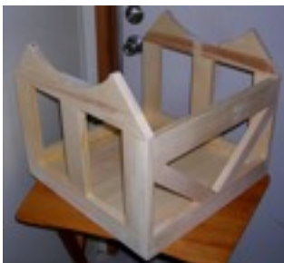
Completed rocker box.
