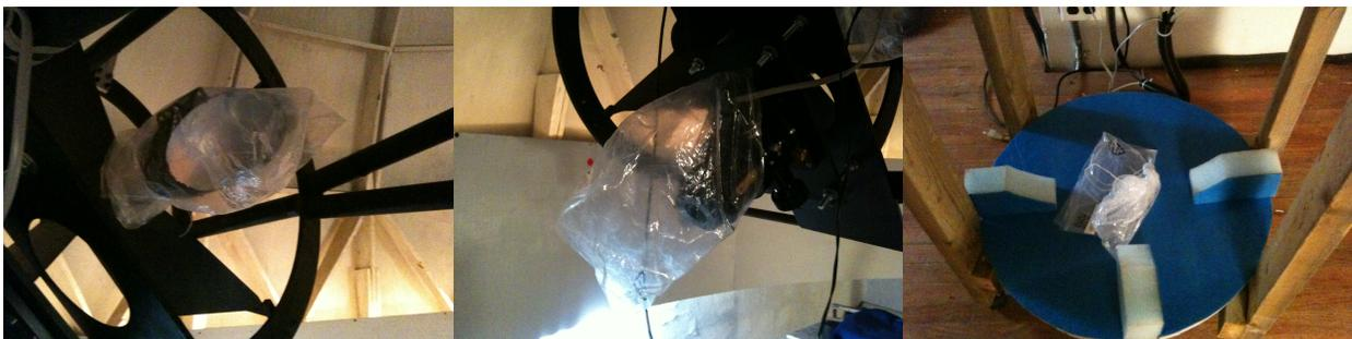
*Figures 15 (Left), 16 (Center), 17 (Right): plastic covers for the secondary mirror (Left) and focuser (Center) are properly stored.*
