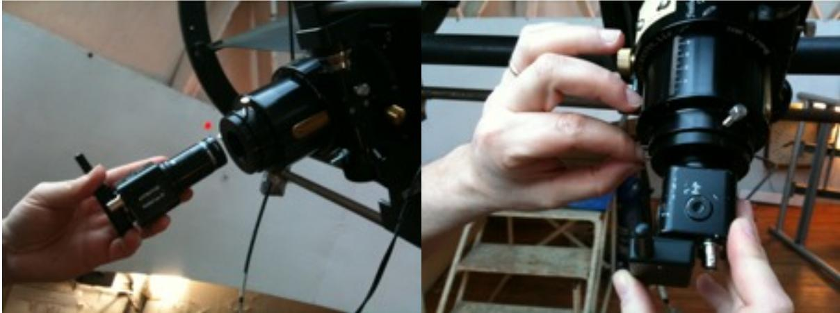
*Figure 18 (Left) and 19 (Right): Camera is secured to the focuser with the antenna pointing up.*
